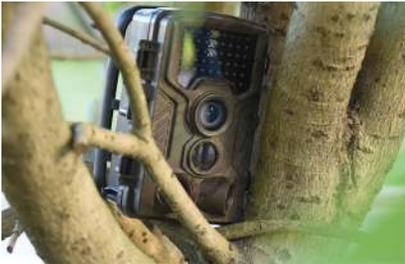
Hunting cameras work using motion detectors. When an animal or person comes near the camera, motion sensors detect movement and take a photo or video.
